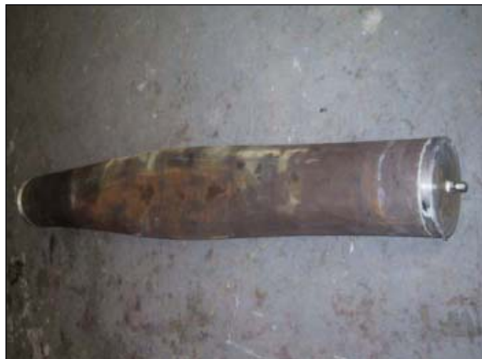
Specimen T2SFE-02 collapsed after exposure to external pressure applied inside a hyperbaric chamber (Fig. 4).
