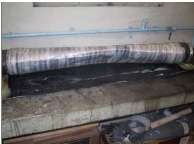
Specimen T2SFE-02 collapsed after exposure to external pressure applied inside a hyperbaric chamber (Fig. 4).
